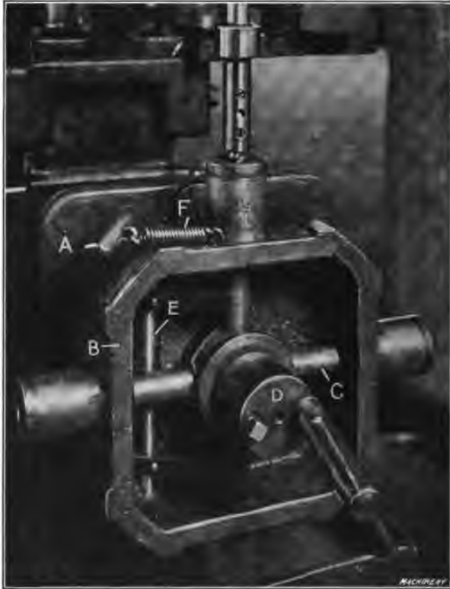
Fig. 12. Indexing Jig provided with Special Work-locating Device
